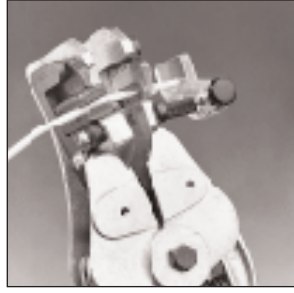
Transparent wire stop provides uniform stripping length.
